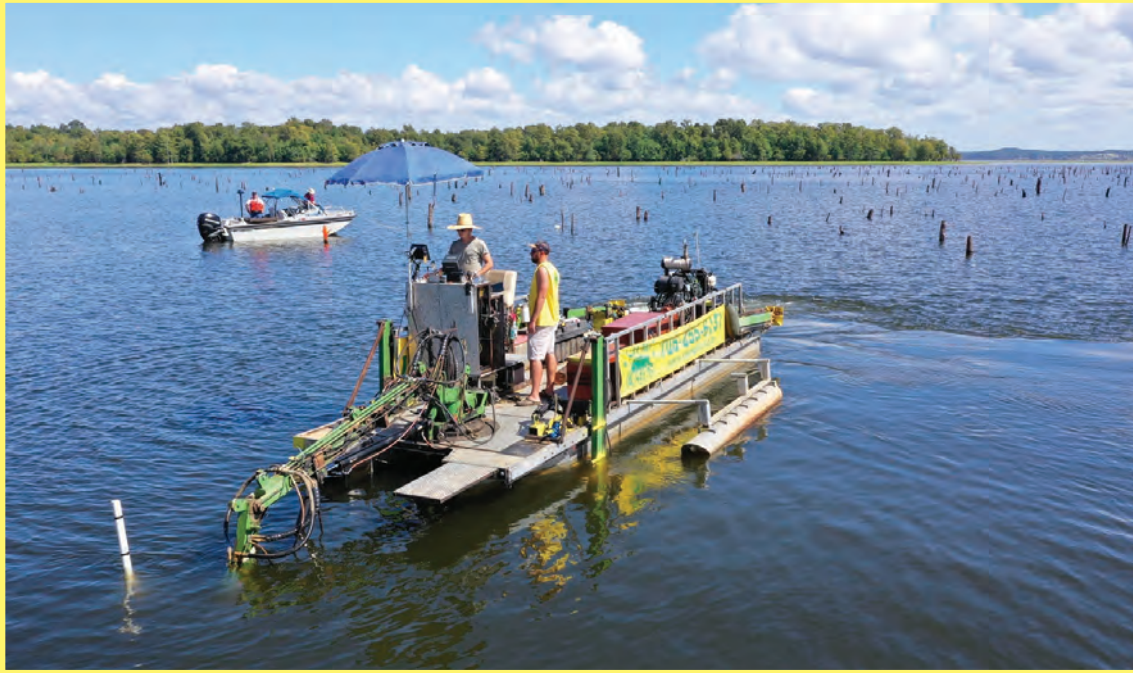
Boat Lane Stump-Cutting Operations
